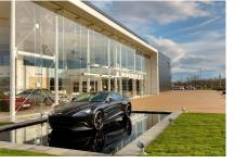
This Aston Martin showroom at Atmell Way, Silver Link in Newcastle shows how impressive sliding doors can look. The installation at this showroom comprised the **record STA 20 DUO** double doors with radar activation and presence sensor for two way traffic. The construction also included battery back-up in case of power failure or fire alarm activation.
