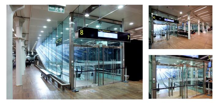
An under floor door drive enjoys a special status. The extra effort required in construction to install the drive unit below ground enables the creation of a free, airy architectural style, and therefore often plays a role in representative glass constructions.
